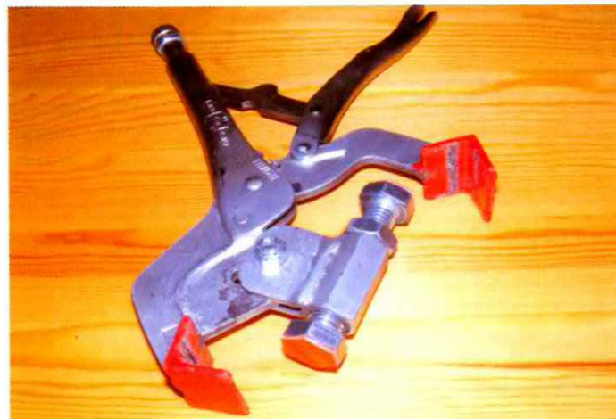
The clamp with the modification of some plastic added to the inner adjusters.
