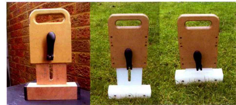
Left to right: The plywood prototype, Polypropylene mallet extended and Polypropylene mallet closed.
